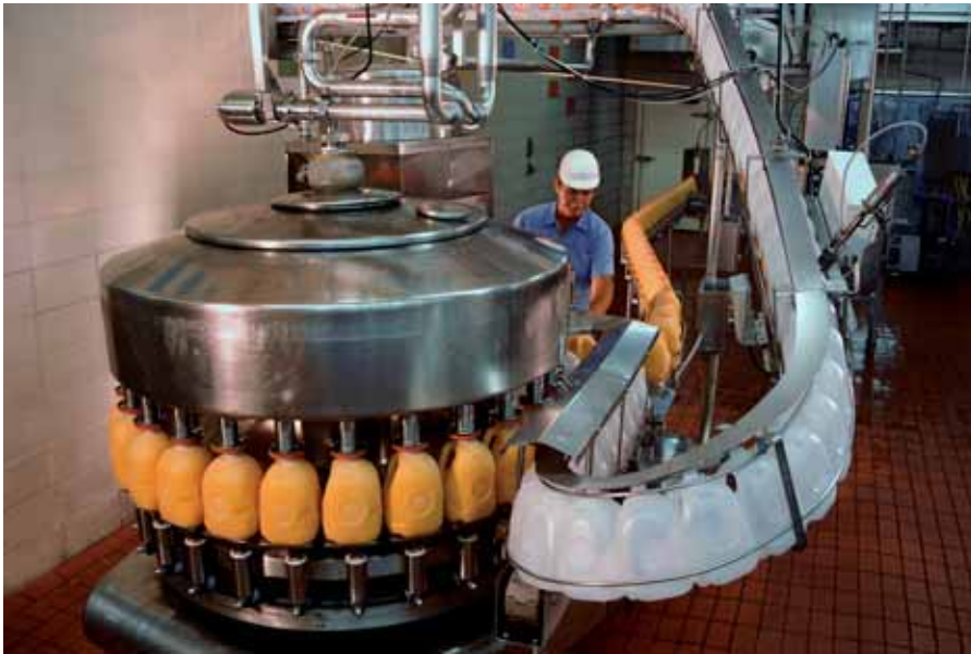
Bottle filling with increased productivity by decreased cycle times thanks to short settling time.
