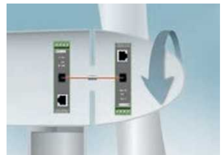
Single-fiber media converters are particularly suitable for bidirectional transmission for rotating applications.
