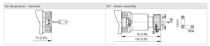
In case of solenoid malfunction or power failure, the spool of the valve can be shifted by manual override. For alternative manual overrides contact our technical support.
