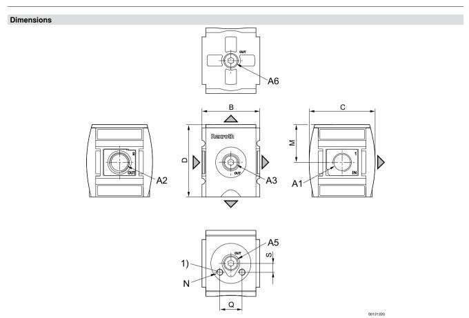
A1 = input A2 = output 1) Mounting thread for pressure sensor
