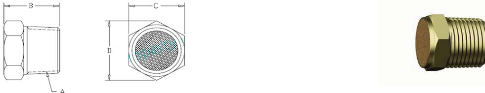
Recommended for pressures up to 125 PSI. Construction brass and bronze. Porosity: 90 micron
