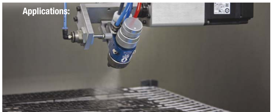
Graco's AirPro EFX™ Automatic Spray Gun automated air-operated application.
