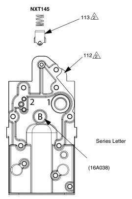
NOTE: To use new detent NXT145 on pre-2009 motors, you must use valve cover 16A038. Order valve cover separately.
