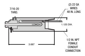
This magnetically operated SPST switch is installed in place of a piston enclosure plug. This "unattached pin" type switch can be used with any size MHH working section An indicator type magnet follows the divider valve piston, opening and closing the switch as it moves back and forth.
