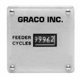
Counter housing clamps to a cycle indicator pin housing. A 6-digit mechanical counter, advanced by the movement of a divider valve cycle indicator pin, provides visual assurance that the system is functioning. Every "count" indicates one complete cycle of the divider valve assembly. Suitable for application at pressures up to 3500 PSI. Part number 563444 (527-002-410)
