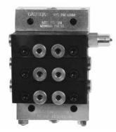
18 through 30 size MHH divider valve sections are available with a factory-installed cycle indicator pin attached to either end of the piston. The pin moves in and out one time for each complete cycle of the divider valve assembly. Application pressure is limited to 3500 PSI.
