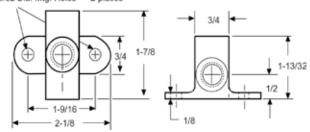
180° Straight Anchor Fitting (plated steel)
