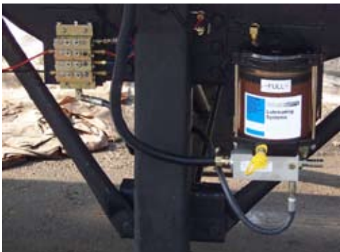
Pump and Divider Landing Gear Mounting
