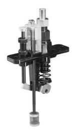
ball is concurrently unseated and lubricant is drawn into the piston cylinder from the sight well. This action creates a pressure reduction (vacuum) in the air- tight sight well, causing lubricant from the reservoir to be drawn into the well until pressure is equalized. On the piston upstroke, the oil in the piston cylinder reseats the inlet shutoff ball and is forced out through the discharge check valve to the machine injection point.
