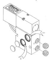
Normally Closed 2-way: Plug Delivery Port #1. Use a Port Isolator to plug internal subbase EXH port. (Internal EXH port corresponds with EXH port in End Cap.) Also plug external EXH port when using Model SBMP-2 subbase, and the appropriate End Cap EXH port. Connect supply pressure to IN.
