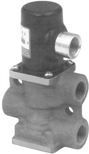
501E1 501E1-3-10-20-36 Model 501E1 is a single-solenoid, maintained-contact, spring-return, 2-way or 3-way valve available either normally closed or normally open.
