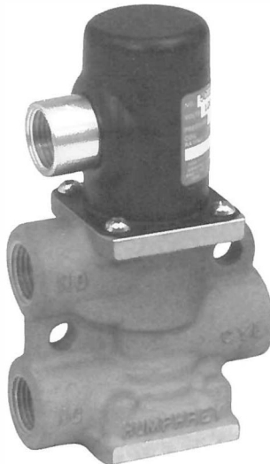
501E2 501E2-3-20 Model 501E2 is a double-solenoid, momentary-contact, maintained-position, 2-way or 3-way valve. If AC coils are to be energized longer than 30 seconds, specify Code CD (Continuous Duty) coils. All coils for DC voltages are Code CD.
