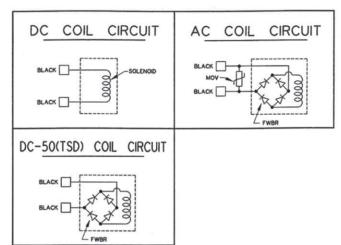
Transient Suppression Diode (TSD), Order code -50, is available for DC voltages to protect drive circuits from DC voltage spikes generated by the valve.
