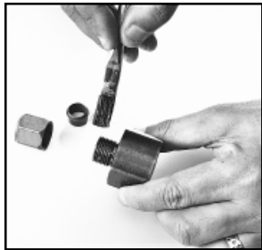
Fig. D7 — Lubricate thread and cone of tool and thread of nut.
