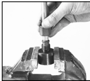
Fig. D10 — Bottom tube end firmly on internal shoulder of Ferulset tool (or fitting body).
