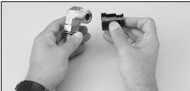
Figure I10 — O-Ring Installation Using CORG Assembly Tool
