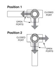
NOTE: Diversion valves do not have off positions, therefore, the center ports can not be used for shut-off purposes.
