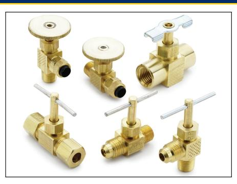
Needle and truck valves have metal-to-metal seats with fine thread screwdown. The lanyard valves' compact design is ideally suited for releasing condensate from air tanks. Brass construction with specially formulated low temperature seal which remains elastic to temperature as low -40°F.
