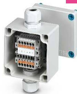
Terminal box with 6 2.5 mm 2 terminal blocks and push-in technology
