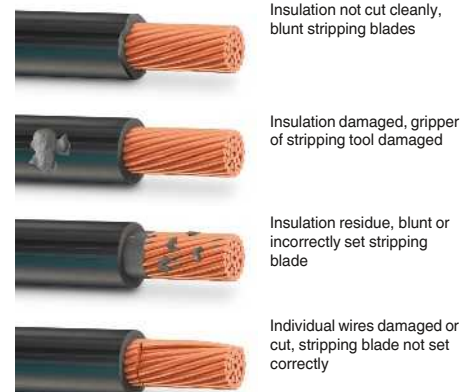
Cable stripped incorrectly according to DIN IEC 60352
