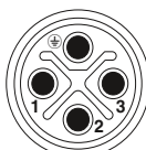
Connector pin assignment of M12 connector, 4-pos., S-coded, view of pin side
