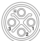
Connector pin assignment of M12 socket, 4-pos., S-coded, view of socket side
