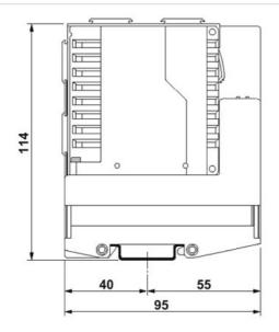
The illustration shows a version of the interface module with the head station FL SWITCH MM  $\ensuremath{\mathsf{HS}}$
