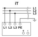
The connection for 3x 400 V AC ... 500 V AC is achieved using the L1, L2, L3 and PE screw connections. The device can be connected to 3-phase systems with nominal voltages 3x 400 V AC ... 500 V AC are connected. In the event of a phase failure, unrestricted operation is possible with nominal capacity. An operation in DC networks is also possible without any limitations.
