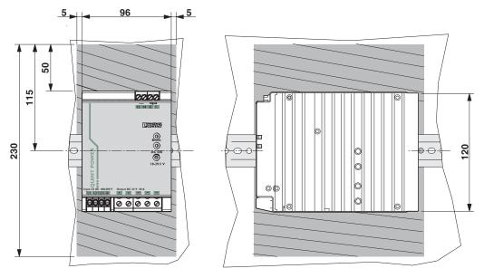
Narrow mounting position: Installation depth 176 mm (+ DIN rail) (default upon delivery)
