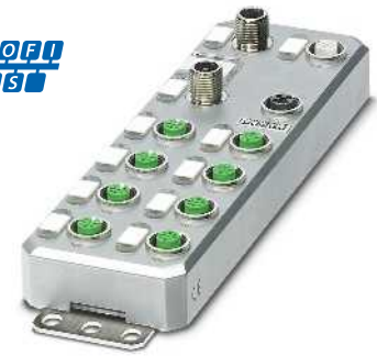
16 configurable inputs or outputs
