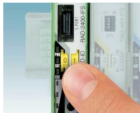
Easy addressing - Only one turn on the thumbwheel of the wireless station
