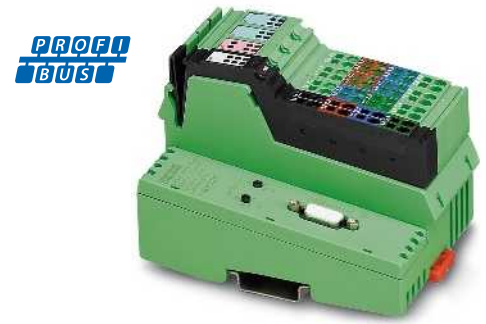
D-SUB connection, 8 digital inputs and 4 digital outputs
