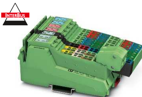
8 digital inputs and 8 digital outputs
