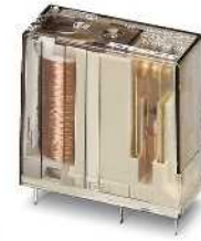
Safety relay with forcibly guided contacts, as per EN 50205, application type B
