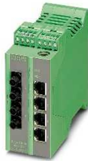
4 RJ45 ports and 2 fiber optic ports in ST format (multi mode)
