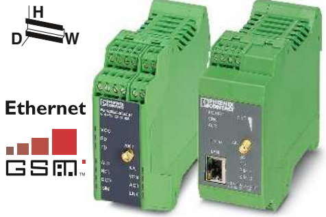
GPRS/EDGE and UMTS/HSPA mobile phone routers for worldwide network access
