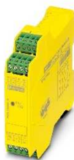
Extension module with 4 additional enabling current paths
