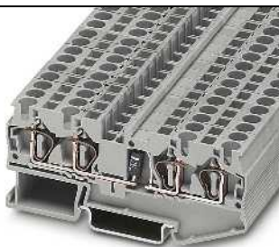
1.5 A, diode terminal block, 1N 5408 (1000 V/1.5 A)
