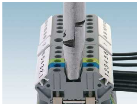
Test finger Ø 12.5 mm
