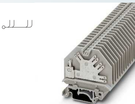
4 (4) mm 2 , 40 A, feed-through terminal block, with screw and slip-on connection
