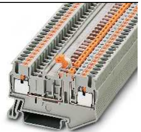
20 A, knife disconnect terminal block, 2 function shafts
