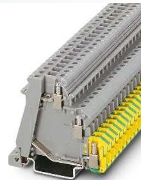
2.5 (4) mm 2 , 26 A, three-conductor actuator terminal block with PE foot
