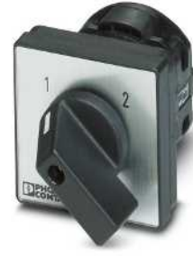
2.5 (2.5) mm 2 , 20 A, switch without 0 setting, with electrically isolated contacts
