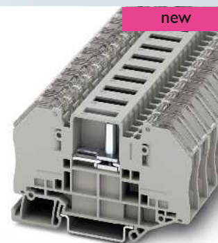
41 A, test disconnect terminal block, with transparent shock protection cover
