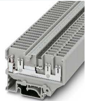
4 (4) mm 2 , 29 A, feed-through terminal block, with screw and slip-on connection
