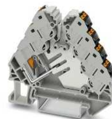
32 A, potential distributor, 11 connections, with supply, can be bridged
