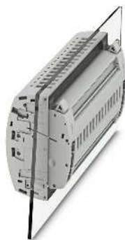
6 (10) mm 2 , 30 A, 4 ... 25-pos. test terminal strip, for wall mounting, screw connection
