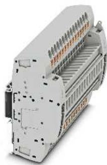
6 (10) mm 2 , 30 A, 4 ... 25-pos. test terminal strip, for DIN rail mounting, push-in connection
