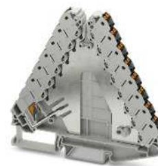
32 A, potential distributor, 29 connections, with supply, can be bridged
