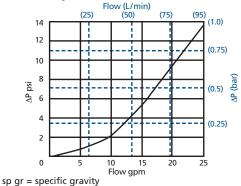
$\Delta P_{element}$ = flow x element  $\Delta P$  factor x viscosity factor
