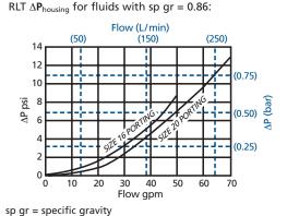
$\Delta P_{element}$ = flow x element  $\Delta P$  factor x viscosity factor
