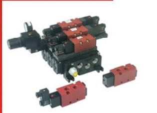
**The C9** is a four-way manifold mounted and body ported, two/three position (5/2 5/3) valve, with 1/2" NPT ports standard and ISO G thread optional. The manifold mounted valves are designed to be mounted on a stacking style manifold and can be electrically operated with a variety coil options, as well as the Plug-In feature. An optional Pre-Wired Amphenol 19 pin connector can support up to 8 valves on a manifold.
