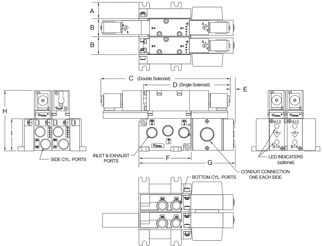
C5, C7 & C9 Stacking Manifolds Dimensions
