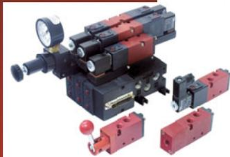
**The C5** is a four-way manifold mounted and body ported, two/three position (5/2 5/3) valve, with 1/8" NPT ports standard and ISO G thread optional. The manifold mounted valves are designed to be mounted on a stacking style manifold and can be manual, pilot or electrically operated with a variety coil options, as well as the Plug-In feature. An optional Pre-Wired sub D connector can support up to 12 valves on a manifold.
