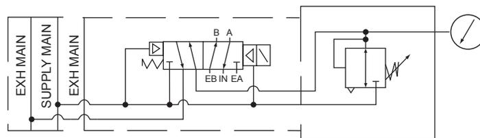
Flow Diagram above shows one single solenoid valve mounted on the Regulator Assembly. Supply Main pressure is supplied to the 'EB' (5) port and Regulated pressure is supplied to the 'EA' (3) port.
