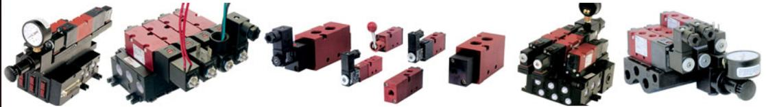
Versa's C-Series, C3, C5, C7 & C9, valves are multi-purpose four-way, 5 port 2 position or 5 port 3 position, pilot operated pneumatic valves consisting of two body types, sideported and manifold mounted. Pilot supply can be either Inpilot or Expilot for all valves with the exception of the C3 which is only Inpilot. A low power solenoid controls the pilot signal which provides the positive force for shifting the valve spool.
