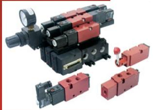
**The C7** is a four-way manifold mounted and body ported, two/three position (5/2 5/3) valve, with 1/4" NPT ports standard and ISO G thread optional. The manifold mounted valves are designed to be mounted on a stacking style manifold and can be manual, pilot or electrically operated with a variety coil options, as well as the Plug-In feature. An optional Pre-Wired sub D connector can support up to 12 valves on a manifold.
