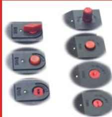
**Overrides** Four types of overrides are available: Standard, Suffix Detail -G, -M and -CML. The standard is a push twist to lock, requires no call out. -G is a guarded momentary contact, -M is an unguarded momentary contact and -CML is a raised grip, push twist to lock.
