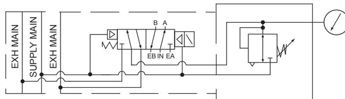
Flow Diagram above shows one single solenoid valve mounted on the Regulator Assembly.
