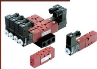
**The C3** is a four-way (5/2) body ported, two position valve, with #10-32 NPT ports standard and ISO G thread optional. It is actuated by single or double pilot (external) or single or double solenoid/pilot (internal). The pilot valve can be used as a five-way valve. A manual override for the solenoid operator is standard.
