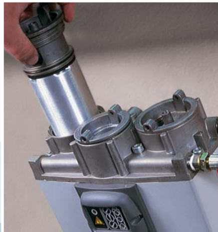
Easy desiccant cartridge replacement
