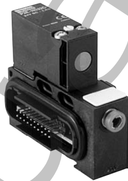
P2S-HW3442CQ 3/2 NC, 5/32", 24VDC, Non-Locking Flush Manual Override & LED Indicator
